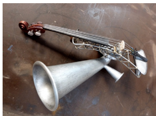
"Song of the Horns" Stroh-violin under construction
